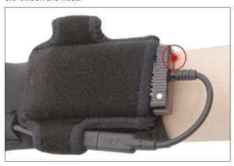
The red light should indicate the gloves are on and warming, they should warm in 15-20 seconds.
