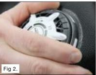
Screw the locking ring onto the dump valve until the valve is lightly held in the suit.
