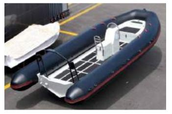
6.0M (19'7) RIB INFLATABLE WITH ALLOY HULL
