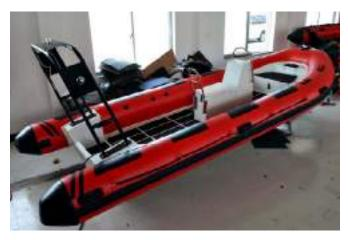
5.5M (18'0) RIB INFLATABLE WITH ALLOY HULL
