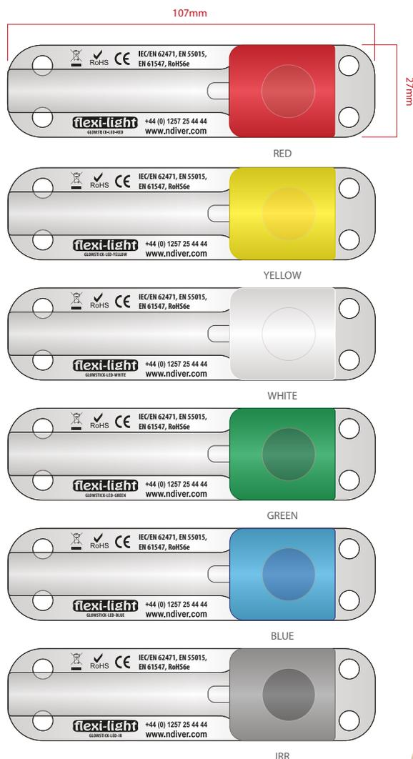
**Flexi-light sticks** have a high intensity LED which projects light through a flexible silicone stick. It has a simple press to operate button under the coloured marker, which activates flashing, constant and off modes.
