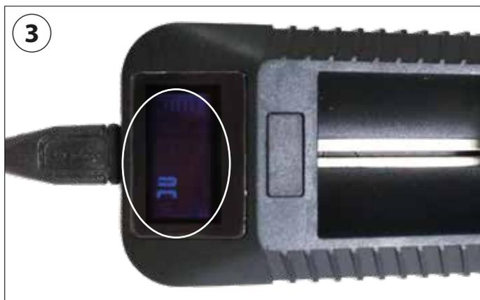
"NC" displayed on the charger's screen denotes that there is no battery inserted or the battery is not charging. The screen may display "NC" for a moment when the battery is inserted. It will then charge normally.
