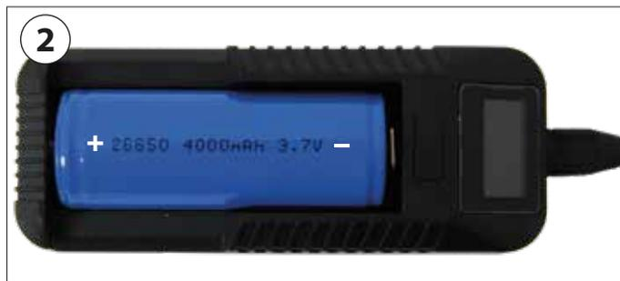
Ensure you insert the battery into the charger the correct way, i.e. with the battery's poles (- and +) touching the corresponding terminals. The correct battery position is labelled on the charger.
