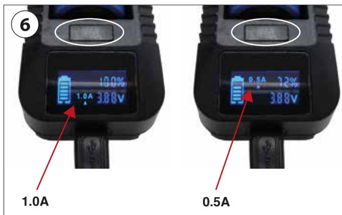
The button above the screen allows you to toggle between a 0.5A current and a 1A current. the 1A current is twice as quick to charge as 0.5A, but the 0.5A current will charge the battery more efficiently and slightly prolong the length of time to the next charge.
