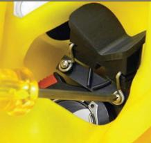
4. Align wire form, block, and pad, then place other screw through the right side as shown. For best results, do not tighten one side completely before the other. Alternate tightening each side.
