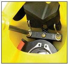
1. First, disassemble the equalizing block and pad by removing the 2 outside screws holding the wire form in place. Remove from GFFM. DO NOT unscrew middle screw.
