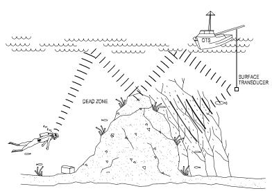
Figure 14: Communication through indirect and direct paths. Note kelp scattering sound. Without surface and bottom bounce, the diver would lose communications.
