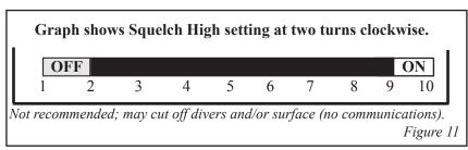
The factory-preset squelch setting is between 1 and 1/2 turns clockwise (or 1/2 turn counterclockwise from full clockwise). If you turn the control two turns clockwise, you will decrease your receive range dramatically, so the divers will have to stay within a few feet of each other
