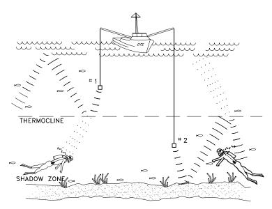
Figure 12: Thermoclines affect the ultrasonic signal. Divers must report thermocline depth(s) so the surface transceiver and/or other divers can be as close to the same depth as possible.
