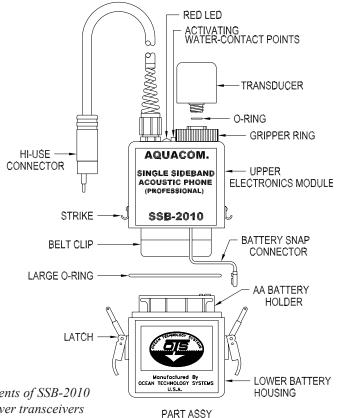
Figure 2. Components of SSB-2010 and SSB-1001B diver transceivers
