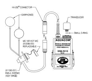
Figure 1. A typical SSB-2010 communication system
