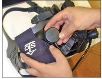
9. The EP-2 earphone is directional. With the shiny side facing toward the diver's ear, insert the earphone into the earphone holder (on each side) past the snaps with the cable positioned below the snap. Secure the snap.
