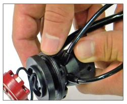
2. Loosen the captive fastening nut on the microphone/push-to-talk (PTT) module of the ear/mic assembly counterclockwise so that there is space between the fastening nut and the base of the module.
