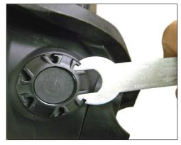
1. Locate the communications port on the right side of the mask. Using the OTS wrench<sup>1</sup> (p/n 137053-000; standard issue with Guardian FFM), unscrew the fastening nut from the plug counterclockwise and remove. The plug is then easily taken out from the inside of the mask.
