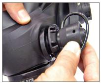
4. Continue inserting the microphone/PTT module into the communications port. The lip of the mask should go over the base of the module and rest between the base and the fastening nut.
