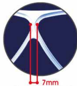
The metal frame attains width of the center portion of frames as only 7mm. It feels like a single lens mask.
