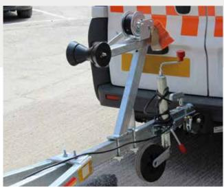
Fully welded and hot dip galvanised, SBS trailers are manufactured this way to ensure they're resistant to corrosion.
