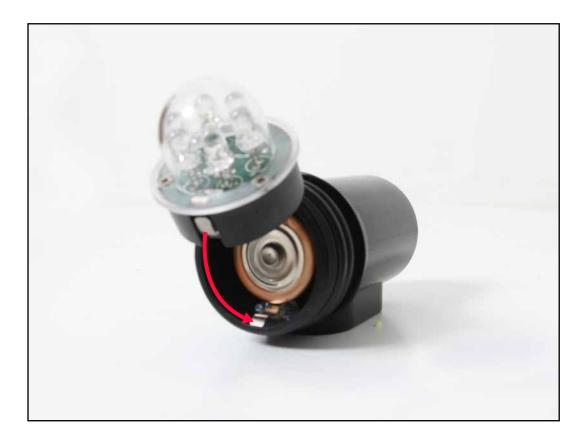
Repeat all the steps in reverse. Going from step 8 to the Step 1 –in order to put it back together, making sure that arrow is pointing down to lock the mechanism when finished.
